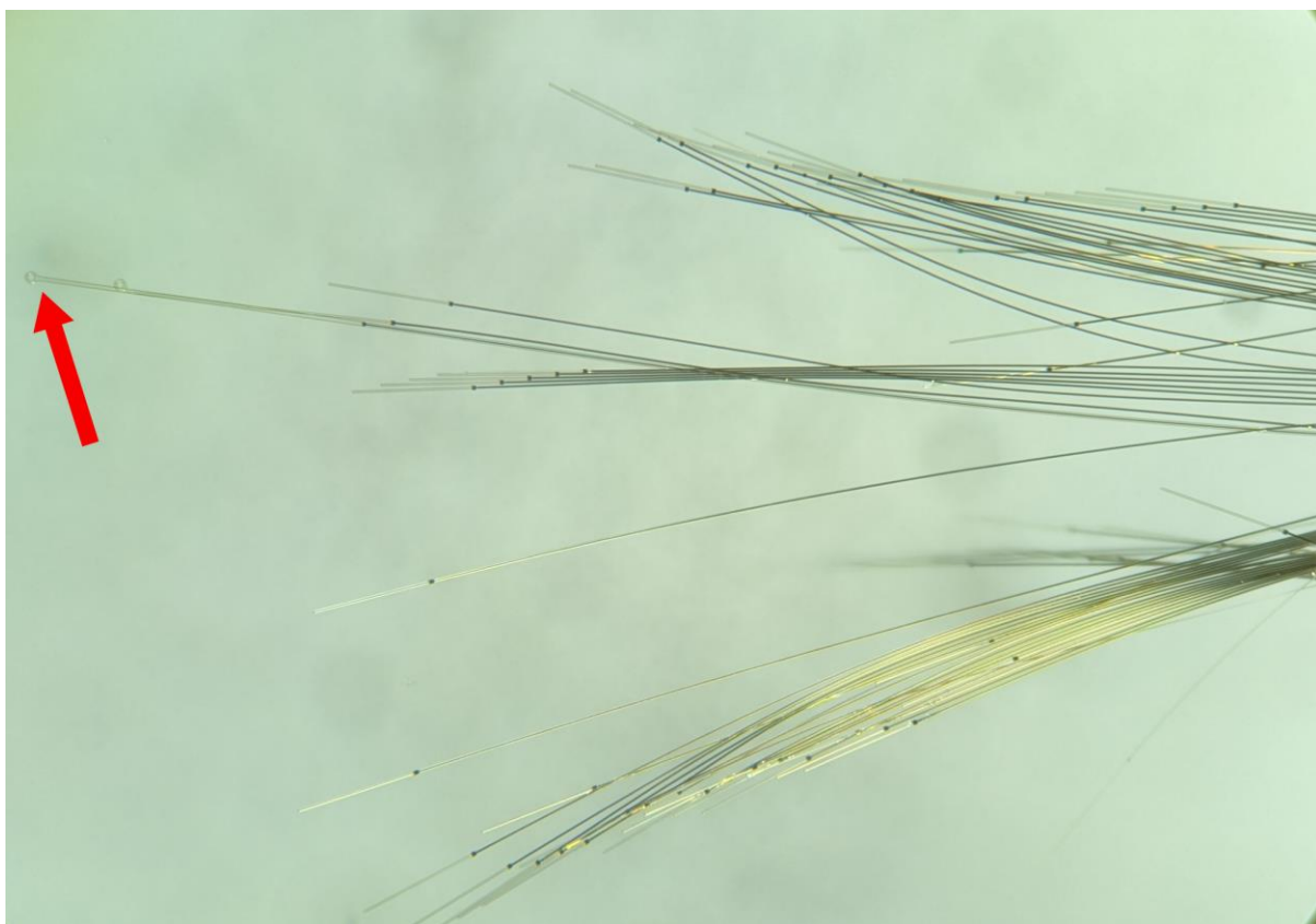
Supplementary Figure 8: A larger version of Fig. 2a(v) showing the electrode fibers of a UFTE bundle floating in distilled water. The red arrow points to the primary loop at the tip of the bundle.
