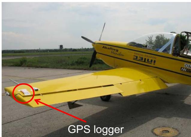
**Figure 11.** Mü30 flight test: Aircraft Mü30 “Schlacro” with GPS logger “GiPSy” mounted on left wing tip.
