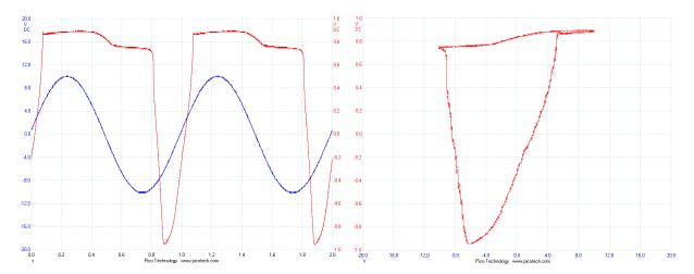
Oxidize silver wire in the 0.5M KCl solution by applying 1.5V to the electrode during 2 minutes (positive output of the power source – to the electrode, negative – to the aluminium bath). Repeat measurement done before (with the Ag electrode). How the properties of the electrode changed? Explain why this has happened. You can get curves similar to pictures below.
